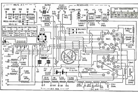
Fig. 2. Schematic circuit of the potentiometer voltmeter.
